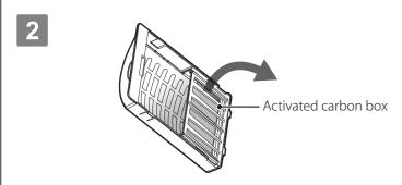
• Pull the activated carbon box in the direction of the arrow.
