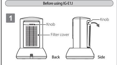
• Hook the knob of the filter cover with your finger and pull outwards in the direction of the arrow.
