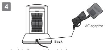
Attach the filter cover to the main body. Then insert the AC adaptor into the main body and plug it in.
